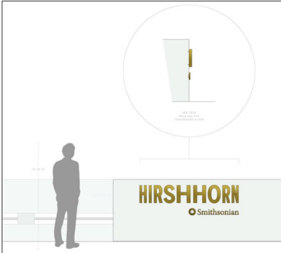
Proposed institutional signage integral to the aggregate concrete perimeter wall at the north and south main entrance overlooks.
