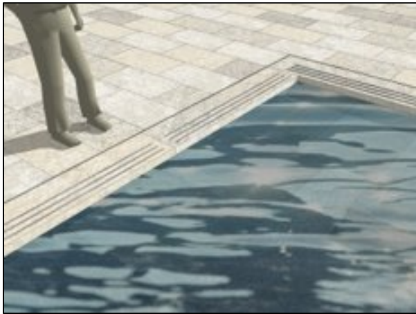
Proposed reflecting pool edge condition with Integral visual and tactile warning units.
