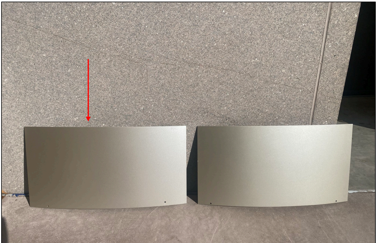
BLC Addition metal cladding finish samples, placed against Colonial Rose granite on the NASM building, February 2025. Selected finish (Titanium) at left, noted with a red arrow.
