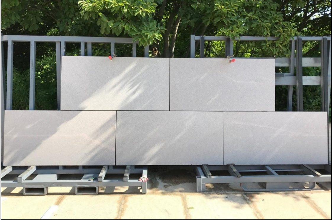
Colonial Rose Granite Mock-up, Sandblast Finish, June 2017.
