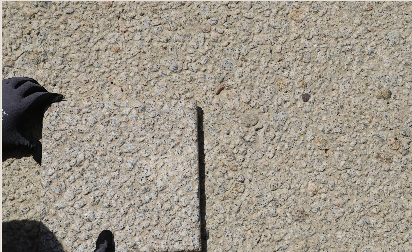
Aesthetic sample of aggregate concrete with Swenson Pink granite, Hirshhorn Museum, 2019.
