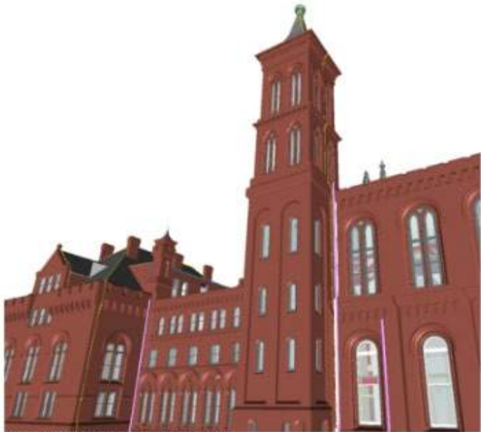
VERTICAL RUN TO GROUND
