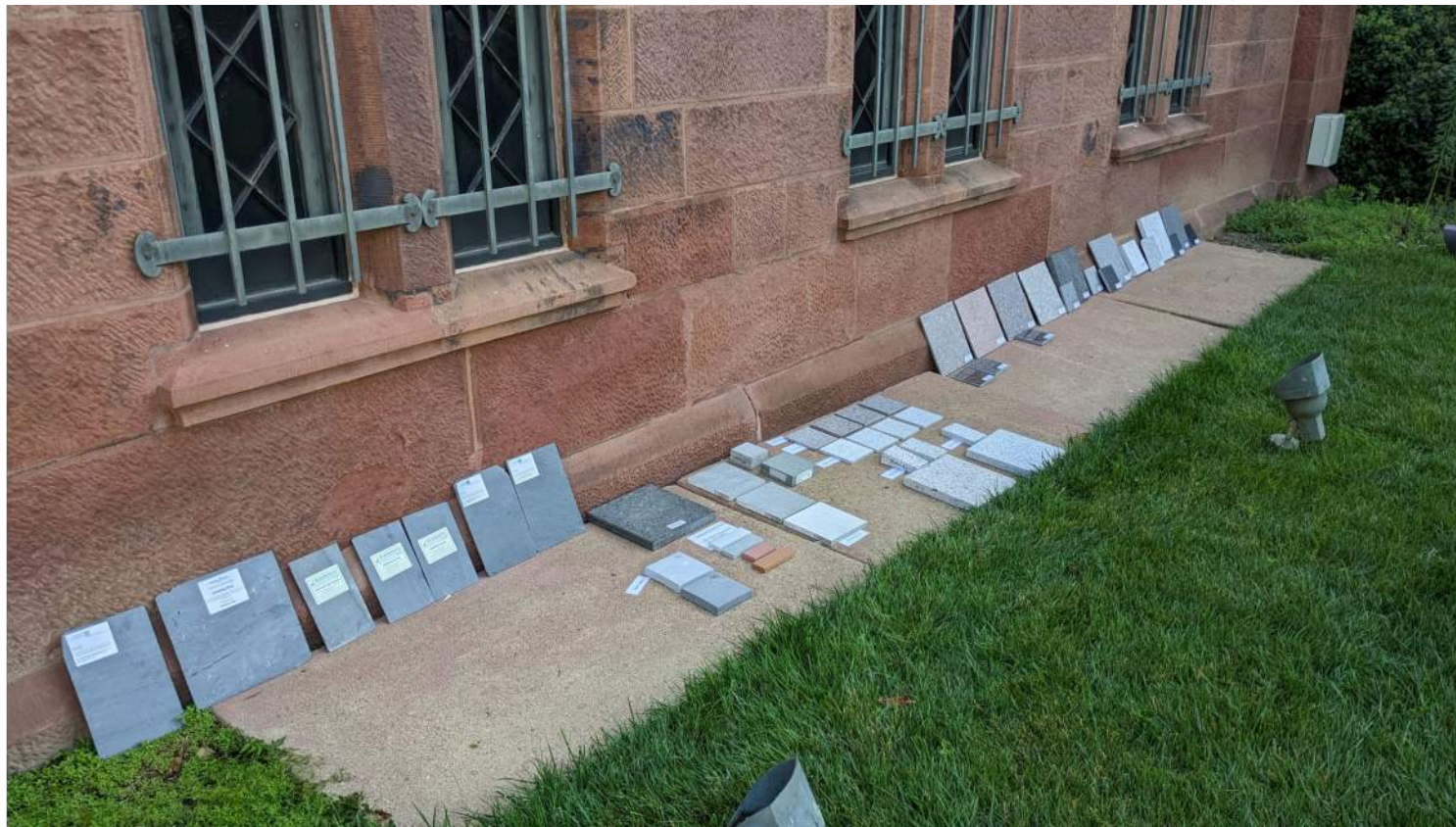
LEFT TO RIGHT: ROOF SLATE, AREAWAY MATERIALS, PERIMETER SECURITY MATERIALS
