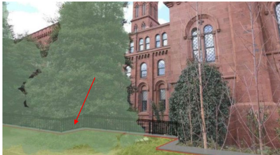
Rendering of the visibility of the Castle's proposed southeast areaway, taken from the Haupt Garden hardscape path. The fall protection railing and plantings will be finalized in Phase 2 of Section 106 consultation. Egress stair gate location is noted with a red arrow.
