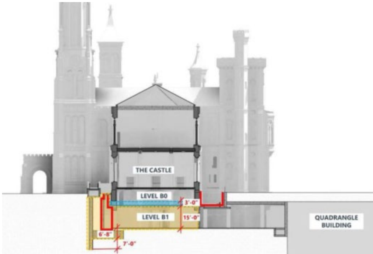
Proposed transverse section through the Castle showing the depths of excavation beneath the Castle. Lowered basement is shaded blue. Mechanical distribution level and seismic base isolation are shaded yellow.
