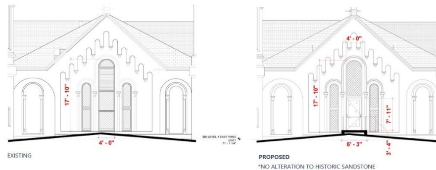
4 th Level Main Building, east elevation. Non-historic window sash will be replaced with a metal and glass egress door with a fixed window above.
