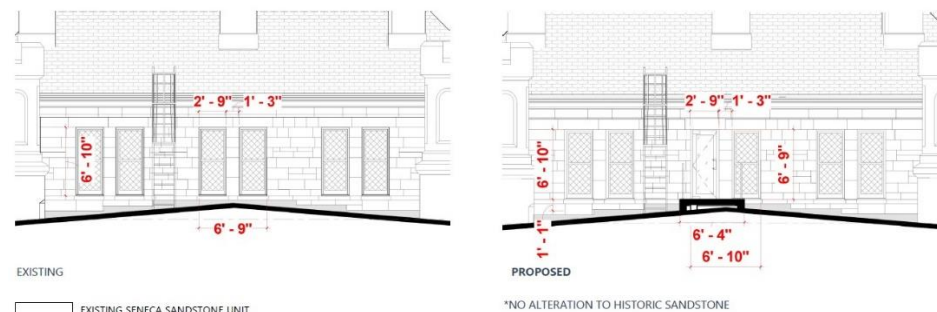
4 th Level East Wing, west elevation. Non-historic window sash will be replaced with a metal and glass egress door.
