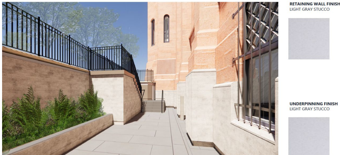
Proposed southwest areaway with gray tinted stucco applied at the retaining walls and the Castle foundation wall.
