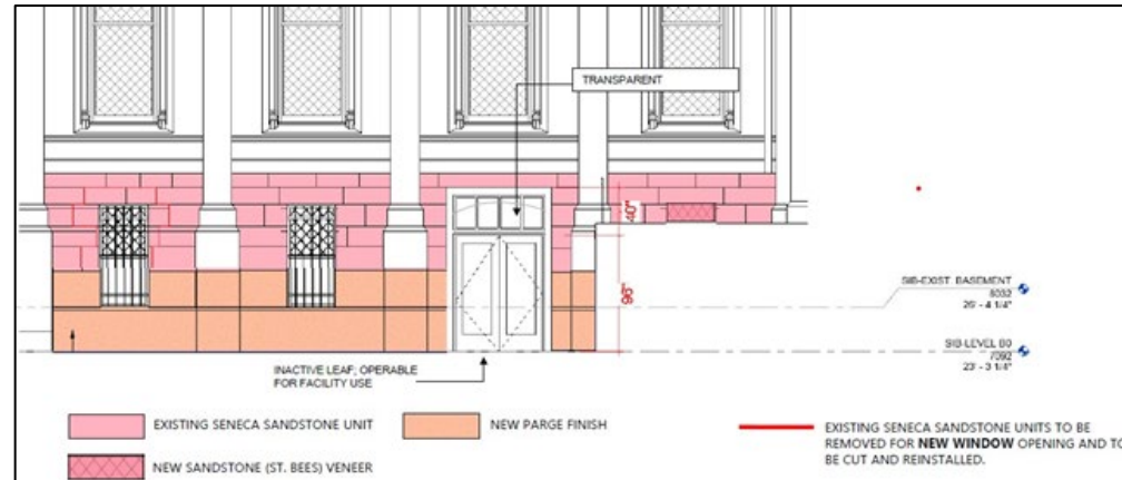
Detail elevation at the southeast basement level with the c. 1871 historic door opening and proposed egress infill.
