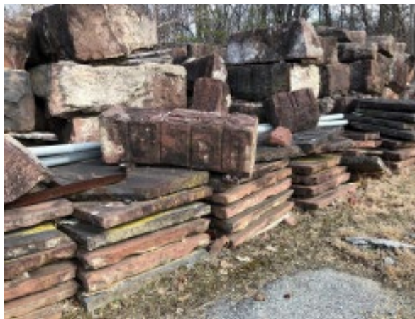
Salvaged Seneca sandstone in SI storage.
