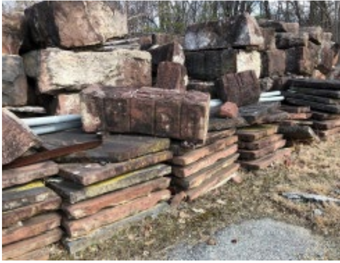
Stipulation 16.A. Use of In-Kind Replacement Materials, Exterior Masonry Repairs to Historic Fabric. St. Bees sandstone sample held against the Castle sandstone at left. Salvaged Seneca sandstone in SI storage at right.
