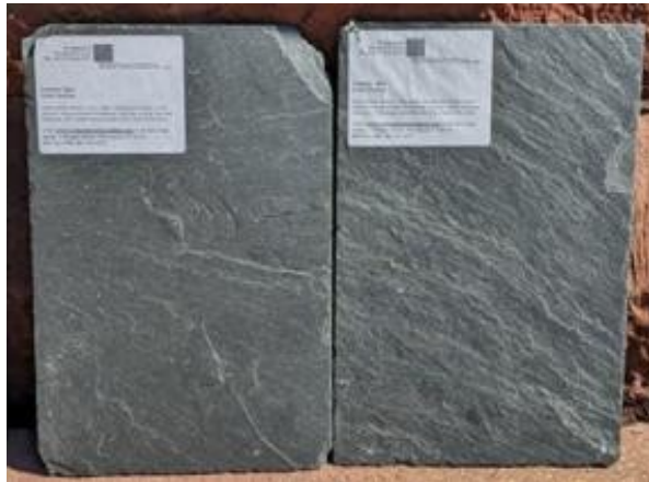
Stipulation 16.A. Roof Materials. Existing Castle slate shingles at left. Proposed Grayson slate shingles at right.
