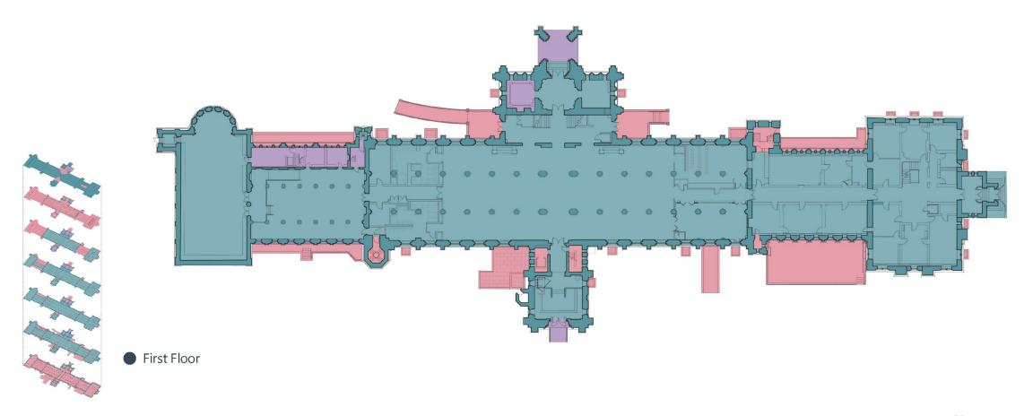
A Historic Structures Report evaluated the building and mapped the exterior and interior into three preservation zones based on the level of sensitivity. Most of the Castle is Priority 1, the most sensitive.
