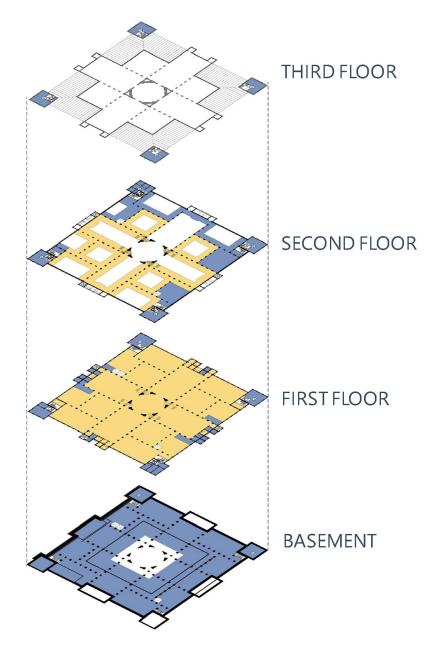
The new basement level will create space for mechanical/electrical equipment and support space for Smithsonian staff. This will allow the historic spaces on the 1st and 2nd floors to be utilized primarily for public functions.
