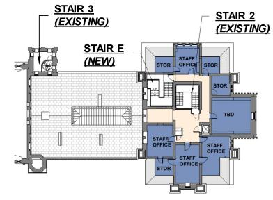
4<sup>th</sup> Floor, Internal Stair Analysis. Stair E is a new insertion that would impact a historic room.
