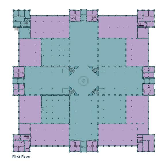
A Historic Structures Report evaluated the building and mapped the exterior and interior into three preservation zones based on the level of sensitivity. Most of the Arts and Industries Building is Priority 1, the most sensitive.
