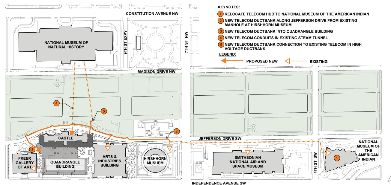
Figure 1.1.2.a - Site plan. Proposed work diagram.
