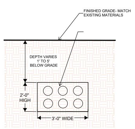
Figure 1.1.3.b - Detail section. Proposed new telecom ductbank.
