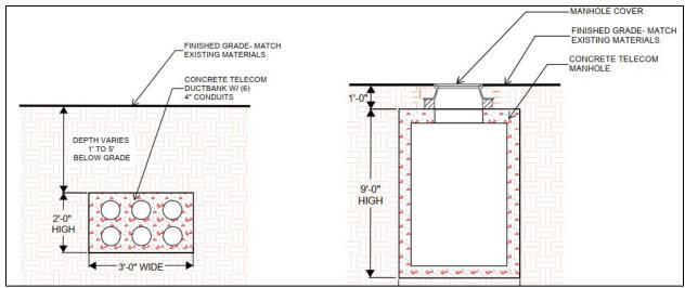
Detail sections of the Telecom Duct Bank and Manhole Access.
