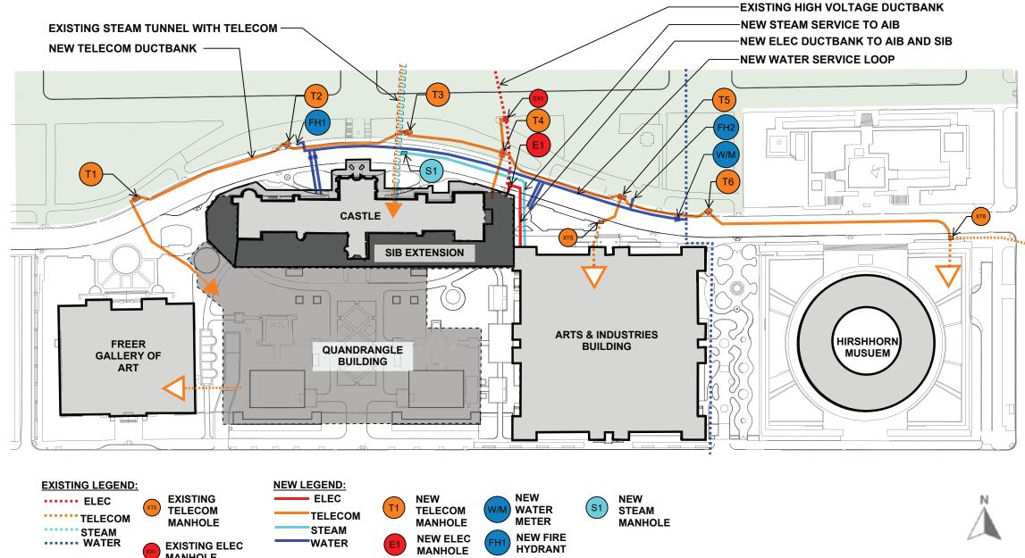
Figure 1.1.3.a - Site plan. New utility work diagram.
