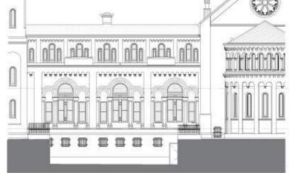
North Elevation of West Range Showing New Egress Door at Proposed Areaway
